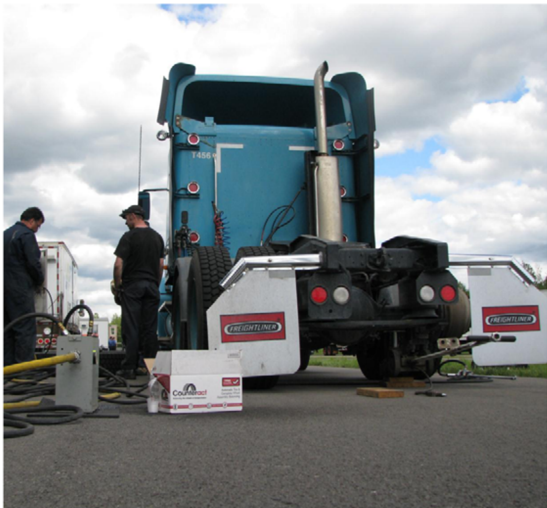
Figure 4. Installation of Counteracting Balancing Beads on the test vehicle.
