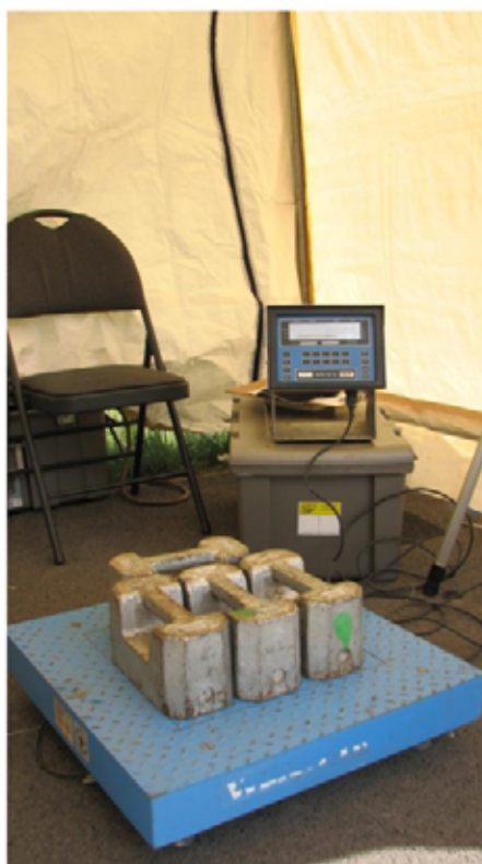
Figure 5. Scale checking using a calibration weight set.
